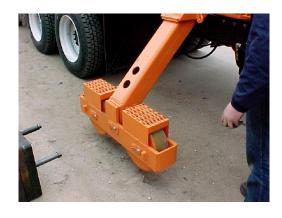
4. The stabilizer is equipped with a manual safety leg. This leg provides additional safety support for the stabilizer. Pivot the safety leg so the pin welded in the lower tube is engaged in the hole at the lower end of the stabilizer. The upper tube of the safety leg is threaded so it can be adjusted to the proper length to line up the holes for the pin. Install the pin. Be sure to install the lock pin and lock it in place.
