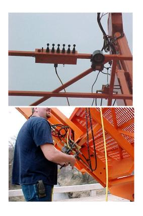
10. Tilt the platform up to horizontal. Operators may now enter platform and attach safety lanyards.
