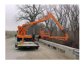
12. With boom #1 horizontal lift pipe to deploy to the platform pipe cradles.
