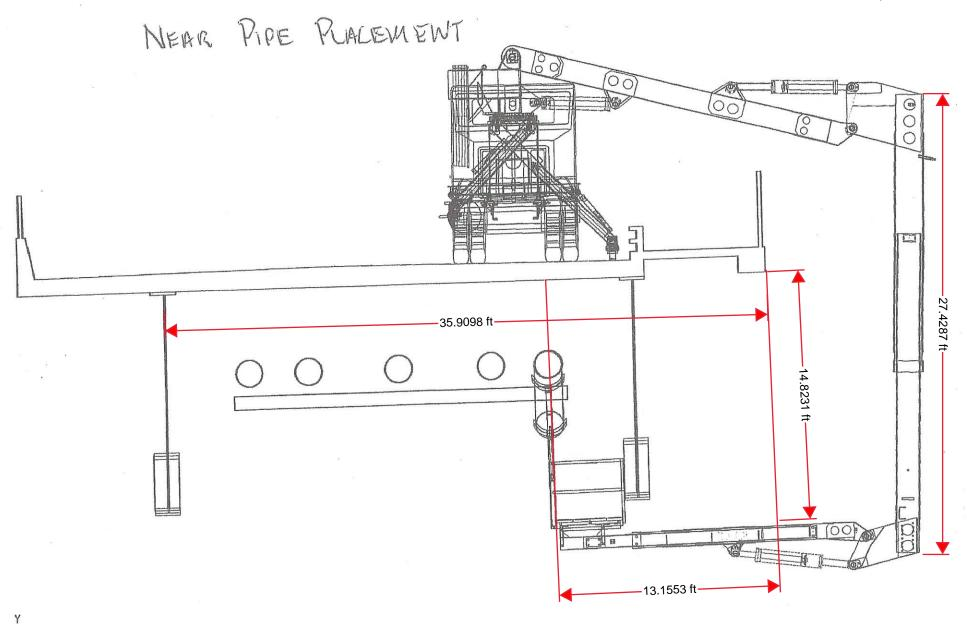
This scenario shows the third boom not fully deployed, but getting a 34' reach from the edge of the deck to the center of the payload.
