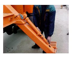
5. At the rear of the bed is the tie down which holds the booms in place for transporting. Remove the tie down at this time.
