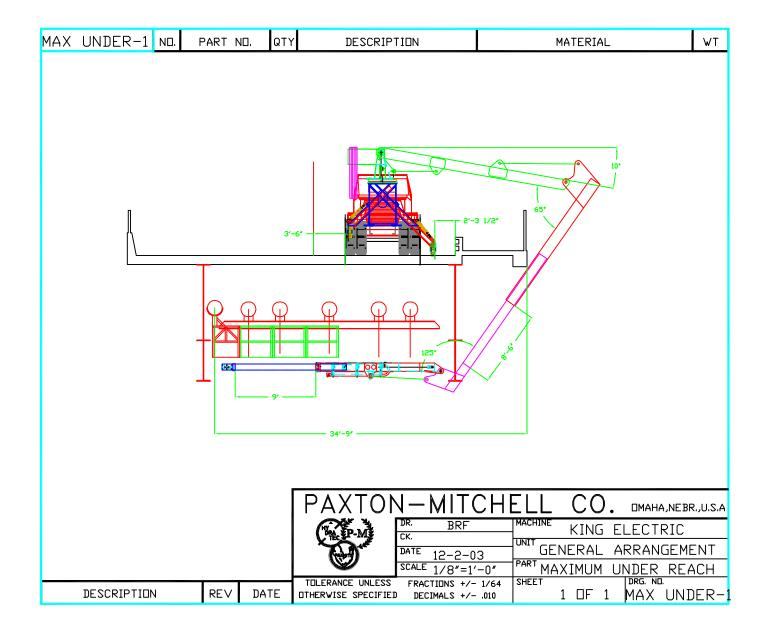
This scenario shows the second boom not fully deployed, but getting a 14'-10" reach from the bottom of the deck to the bottom of the platform.
