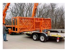
8. Tilt boom #3 down and telescope out to attach platform.
